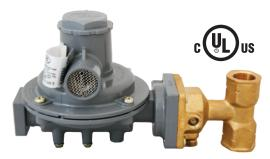
**MEGR-1232T Compact Series:** Offers a compact integral two-stage regulator design perfect for lower BTU applications and confined spaces. They feature an adjustment range from 9-13" WC (factory set @ 11" WC). Stainless steel integral components, fluorocarbon (FKM) seat discs, molded lip fabric reinforced diaphragms, and large precision machined aluminum orifices providing superior downstream regulation and maximum corrosion resistance against weather or contaminated gas.
