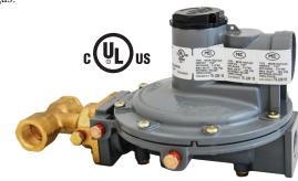
**MEGR-1632 Full Size Series**: Offers all of the same features as the compact MEGR-1232 series in a full size high capacity version. The full size MEGR-1632 diaphragm provides superior downstream regulation, has heavy duty wrench flats and a large 3/4" FNPT tapped drip lip vent to help prevent relief vent blockage.
