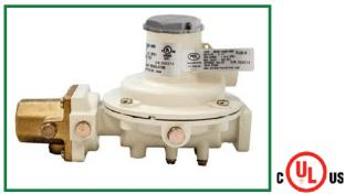
**MEGR-1232E Compact Series:** Offers a compact integral two-stage 2 PSI regulator design perfect for lower BTU applications and confined spaces. They feature an adjustment range from 1-2.2 PSI (factory set @ 2 PSI). Stainless steel integral components, fluorocarbon (FKM) seat discs, molded lip fabric reinforced diaphragms, and large precision machined aluminum orifices providing superior downstream regulation and maximum corrosion resistance against weather or contaminated gas.
