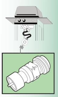
**CAUTION:** The disposable cylinder must always be within 45 degrees of the upright (vertical) position when connected to the grill connection. Failure to do so can result in LP in its liquid form entering the grill. This could result in explosion, fire hazard or personal injury.
