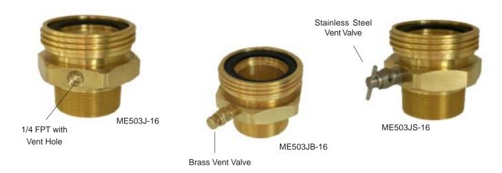
Vent valve purpose is to safely discharge excess vapor and liquid trapped in the line before disconnecting the transfer hose. Commonly used on bobtail and transport vehicles.
