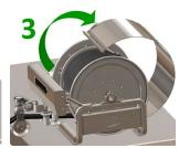
To remove the cover -Pull both detent pins, push the cover to the left to release it, and lift it upward. Latch and pin cover when done.
