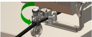
2. Press and release the "REEL OUT" button on the PC3 or ASKW and keep remote with you.
