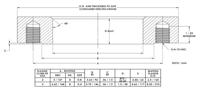
FIGURE 1: TANK FLANGE DIMENSIONS
