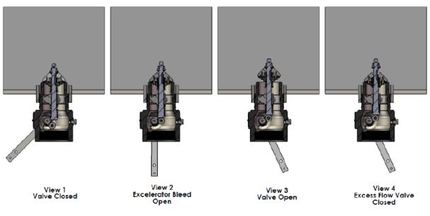
Figure 1: Operational Schematic
