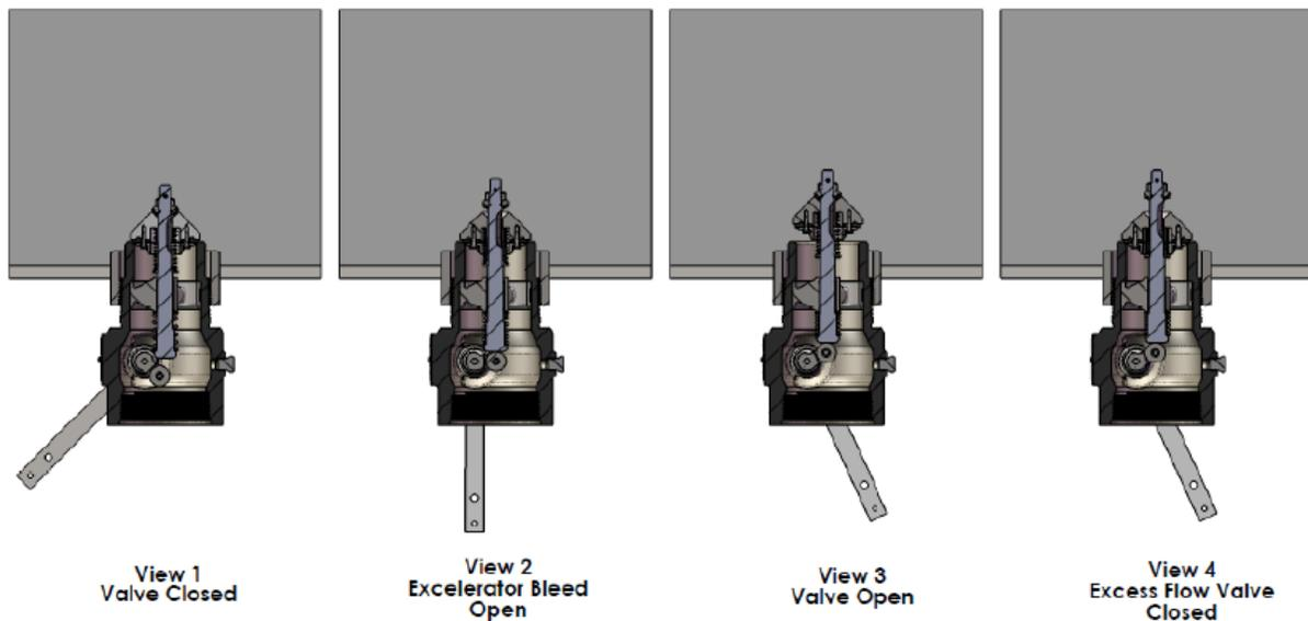
Figure 1: Operational Schematic
