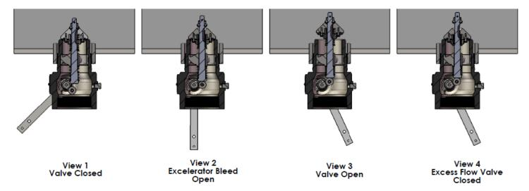
Figure 1: Operational Schematic
