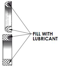
10. Install Stem O-Ring [3b], Female Adapter [3c], (2) V-Packs [3d], Bushing O-Ring (cut) [3f] and Male Adapter Bushing [3e] into Valve Shaft Gland [3a] as shown.
