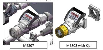
4. Connect a pressure source of a least 150 psi (1034 kPa) and check for leaks (as evidenced by bubbles) at all joints and sealing surfaces, using a suitable leak detector solution at all joints. Ensure all connection joints are free of leaks before putting the ME807 or ME808 LE valve into service.
