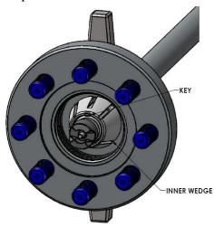
7. Install Outer Wedge into Flange Adapter and tighten securely. Tighten Set Screws securely.
