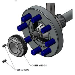
8. Install Key Retainer into Mounting Flange as shown.
