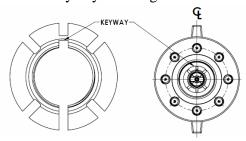
6. Install key until flush with Inner Wedge.
