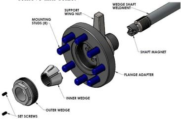
2. Install Wedge Shaft Weldment through tank and Flange Adapter.
