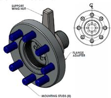
3. Apply good quality pipe sealant to NPT threads of Flange Adapter. Thread Flange Adapter, with Support Wing Nut fully installed, into tank coupling using MEC installation tool MEP930WG, tighten securely. Centerline mount Flange Adapter. Tighten Support Wing Nut securely against tank coupling using MEC installation tool. Flange must be centerline mount to prevent error.
