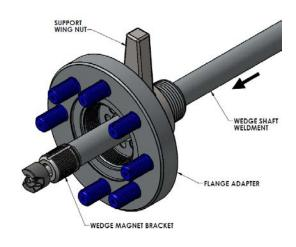
4. Install Inner Wedge onto Wedge Shaft Weldment until Inner Wedge stops.
