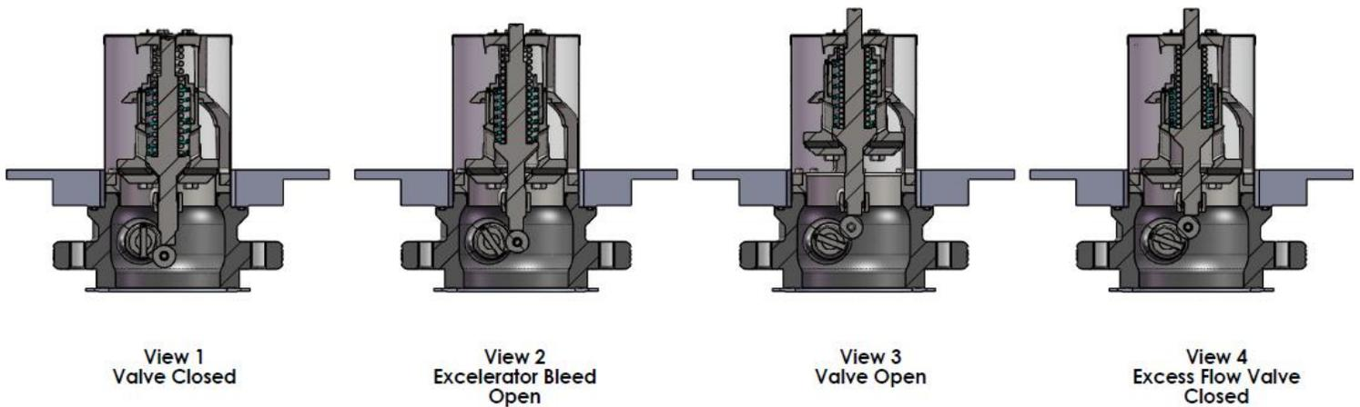
**FIGURE 4: Operational Schematic**
