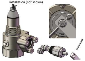
The valves feature a break off section located below the inlet pipe thread which is intended to permit the lower valve body to shear off in an accident, leaving the valve seat in the tank. The break off section is designed for container installations and may not provide shear protection if the valve is installed in a pipeline.
