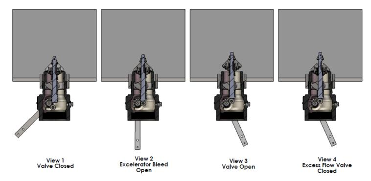
Figure 1: Operational Schematic
