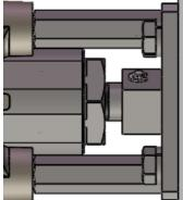
6. Connect the actuator pressure line tubing to the inlet port. After installing the unit, operate the actuator with pressure to confirm it smoothly opens and closes the internal valve without sticking or jamming. Confirm actuator opens the valve a full 90 degrees by watching the indicator lines.
