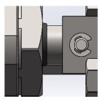
**For Fisher® Valves ONLY:** Remove the screws holding the cover plate to the internal valve body, discard the screws and retain the cover plate. Ensure that the internal valve packing rings remain in position during disassembly and reassembly. With the cover plate in position, install stand-offs [4] through cover plate and hand tighten.
