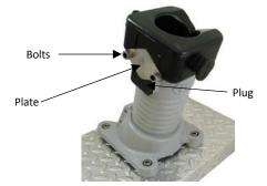
b. Insert the sensor paddle into the slot in the receiver as shown, reinstall the (2) bolts and tighten securely.
