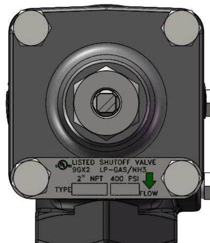
Angle Valve Nameplate Orientation
