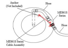
Use a short length of hose between the rigid piping and the inlet of the pull-away valve. Confirm the short length of hose is long enough to allow the pull-away valve to bear the brunt of any excessive tension load in the event of a pull-
