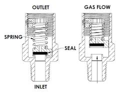
Initial discharge may be small, producing only seepage and a light "hissing" sound. As discharge pressure and volume increase, a "popping" condition or a continuous "hissing or roaring" sound will occur.
