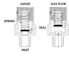
Initial discharge may be small, producing only seepage and a light "hissing" sound. As discharge pressure and volume increase, a "popping" condition or a continuous "hissing or roaring" sound will occur.
