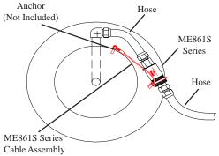
Use a short length of hose between the rigid piping and the inlet of the pull-away valve. Confirm the short length of hose is long enough to allow the pull-away valve to bear the brunt of any excessive tension load in the event of a pull-away.
