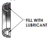
5. Install components from Step 4 into Valve Shaft Gland [12] as shown.
