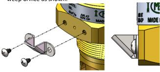
Replace protective cap onto relief valve.
