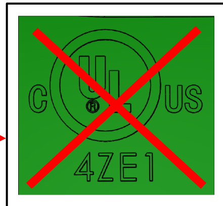
6. Install Dust Cap into Body. Deface UL Logo and Barcode on Body.
