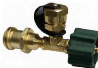
1-5/16" Male ACME w/ Quick Closing Poppet x 1-5/16" Female ACME x Male 1" -20 Bulk# ME418 Packaged# ME418P
