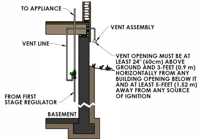
Figure 4: Basement Installation
