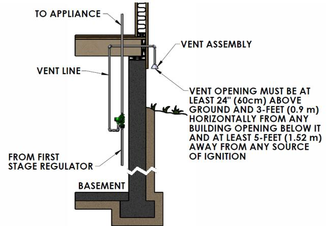
Figure 4: Basement Installation
