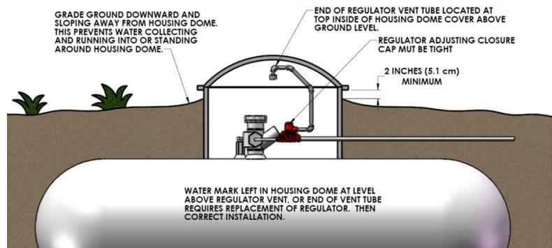
Figure 5: Underground Installation
